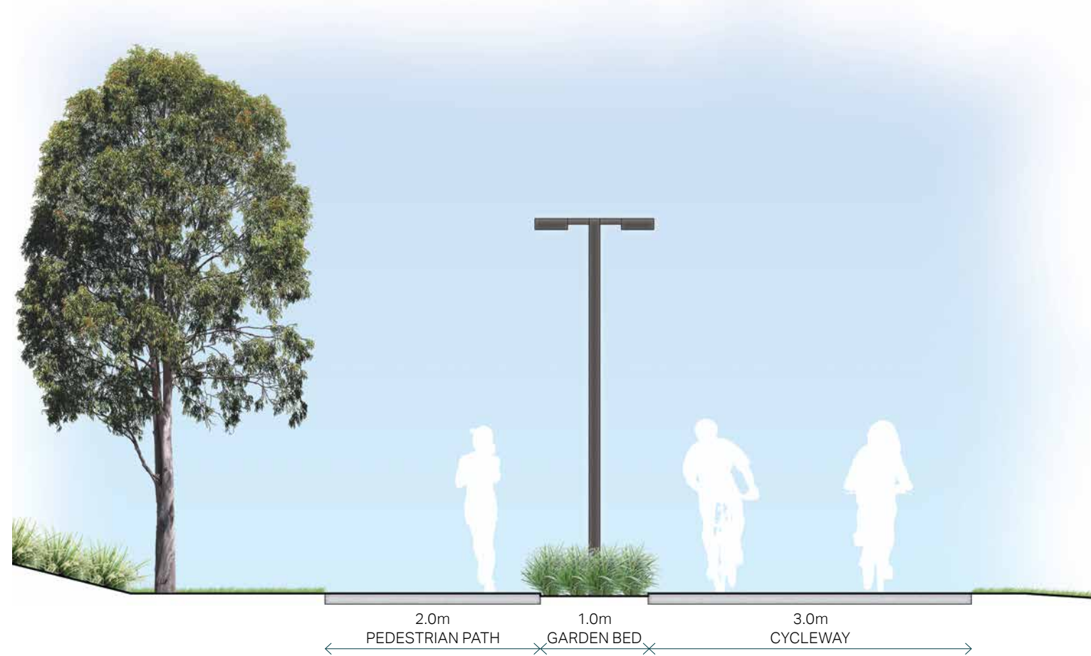
DETAIL AREA: PARRAMATTA VALLEY SEPARATED CYCLEWAY 1:50@A3
