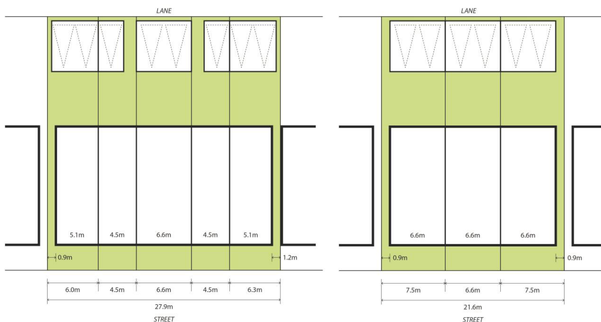
Figure 3-4. Two examples of lot subdivision for 'sets' of attached or abutting terraces
