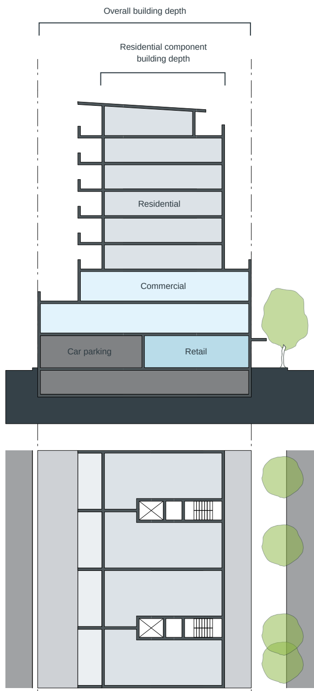
Figure 2E.1 A mixed used building showing the transition of building depth: deeper floors on lower levels dedicated to retail/commercial uses and narrower residential apartments on upper levels
